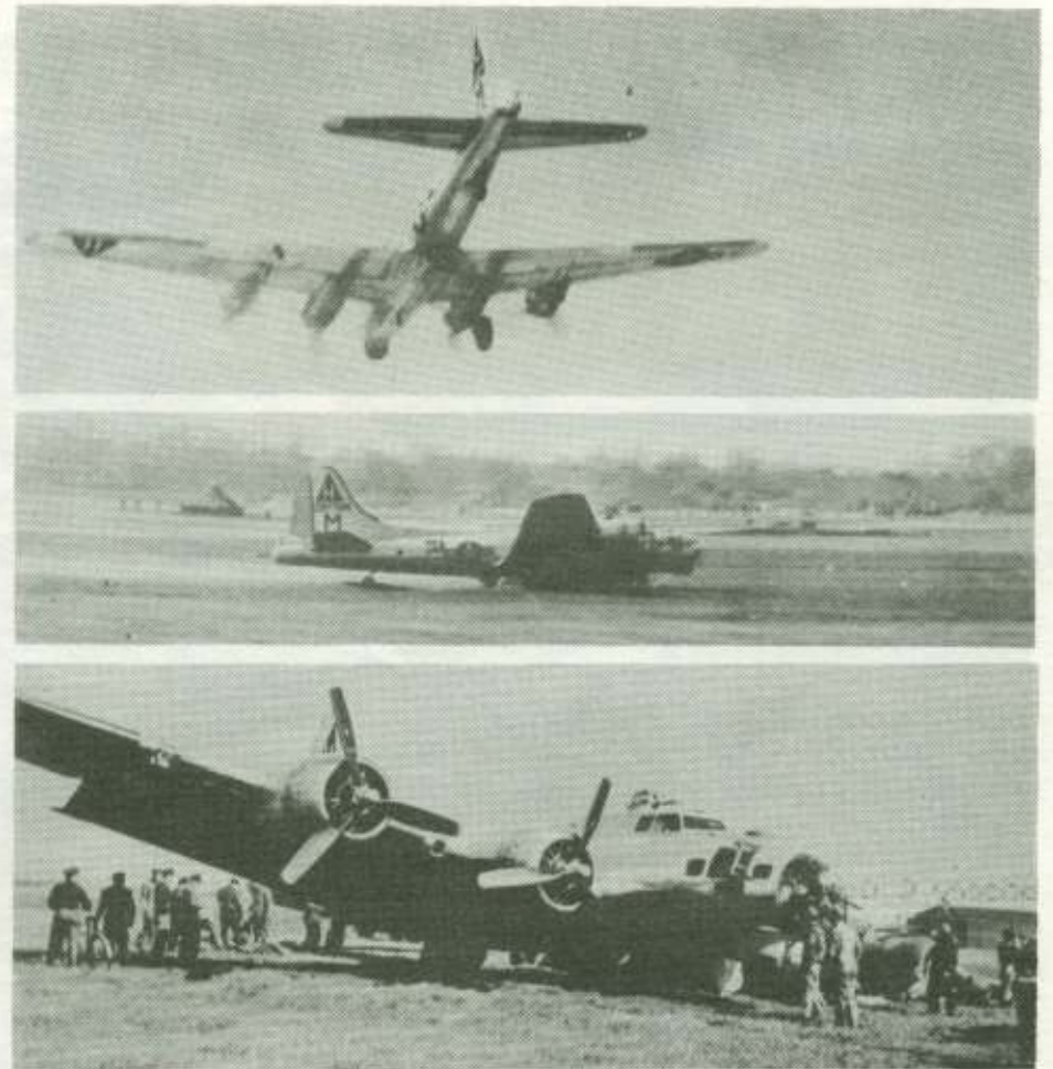
Fortunate Youth arrives 25 Apr 44 at Thurlleigh for assignment to the 369th squadron and to the crew of Lt. Clifford Baxter. He and his crew had arrived 12 April, and had a couple of missions before being assigned to this aircraft. A raid into France on a Noball target brought a flak-induced rupture in an oil line and the left wheel would not drop. After flying around four hours to reduce the gas load, they came in alongside runway 06 to land. The plane was put back into flying condition, with a new wingtip and two new engines in a matter of 28 hours. Fortunate Youth was burned 7 Aug 44 when a cockpit fire in 086 was followed by an explosion that destroyed the two airplanes. Who was the ground crew chief?
